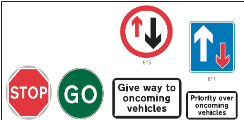
Figure 1.7: Manually operated stop/go signs and priority signs.
